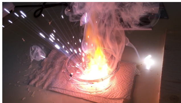
Fig. 9. When cool water was thrown over the melted grains of lithium within a glass bowl, a lithium explosion took place that lasted approximately three seconds. The photograph shown is from a video shot at a frame rate of 240 Hz. The white hot lithium plasma is at the bottom of the explosion and pieces of plasma are blown out as coulomb explosion white hot fragments. The orange fire on top forms lithium oxide and/or hydride colloidal particles which then go up in smoke.
